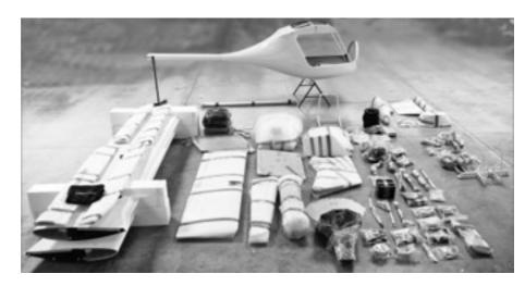
As standard S kit plus MTOW 520kg wings(complete), Steel MLG Legs
